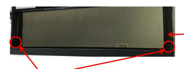
Unscrew two screws on each side and then take off two bars that covers the visual glass.
