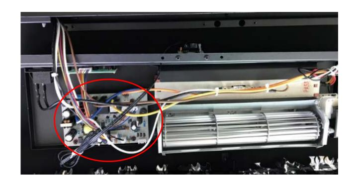
Unscrew 4 screws and then you can take the PBC board from the set and replace it with a new one.
