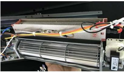
Unscrew 4 screws and you can remove the heating element from the set. Now you can replace it with a new heater.
