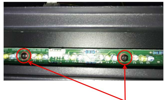
The ember bed LED light bars are fixed by <u>screws</u>, unscrew the screws to take off the LED bars and replace them by new ones.
