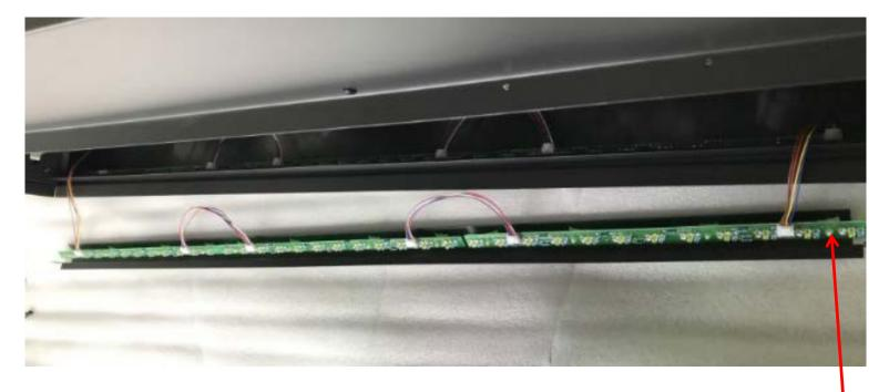
After STEP 3 you can take out the whole flame effect LED bars assembly and each LED bar connects with the assembly via a plastic fixer. Get the LED bar from the fixer and replace a new one.
