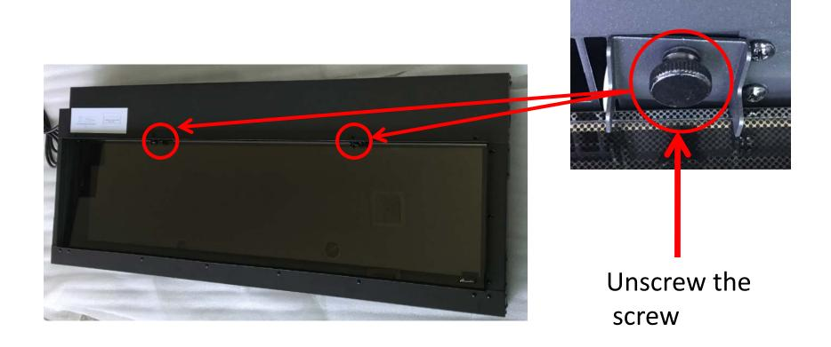
Unscrew one screw on each side and then remove the front glass.
