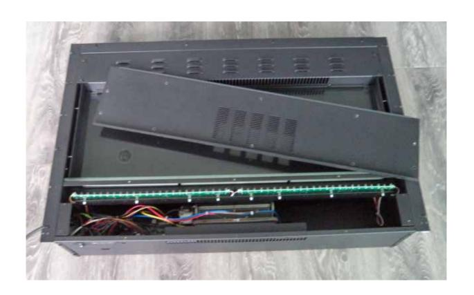
3.Unscrew screws at the both sides and the top and take off brackets. Then carefully remove the back glass from the unit.
