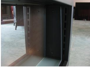
Unscrew two screws and take off bracket both side.
