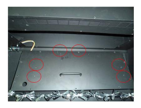
Unscrew 6 screws and take out the bad heater. Replace a new one. Plug the internal wire back and screw back all the part.
