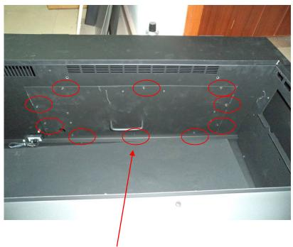
You can see the top panel. The part show at the picture. Unscrew 10 screws. Using the handle, lift the panel away from the unit.
