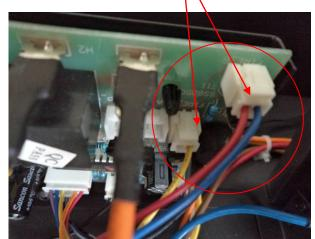
To check if the PCB board is working, switch the positions of the wires as shown.
