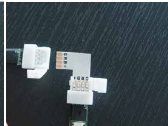
Detach light strips from Corner connector
