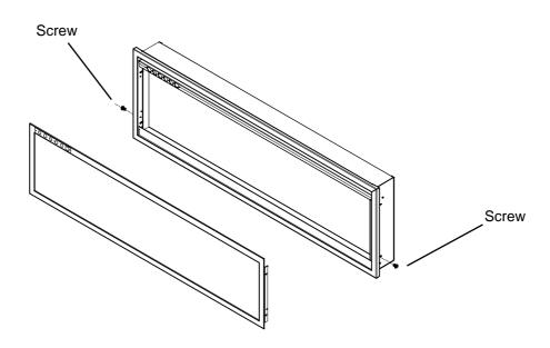
2. Unscrew the 2 screws located on each side and take off the inner side steel panels.
