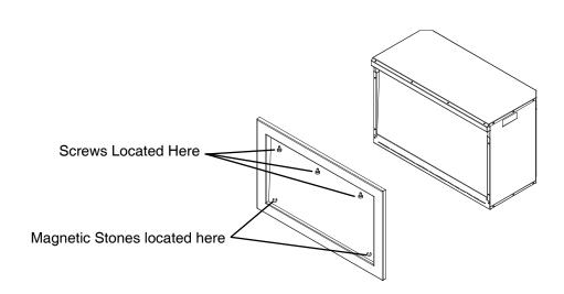
2. Carefully remove the front glass panel once the trim has been removed. Use caution as the glass is now loose.
